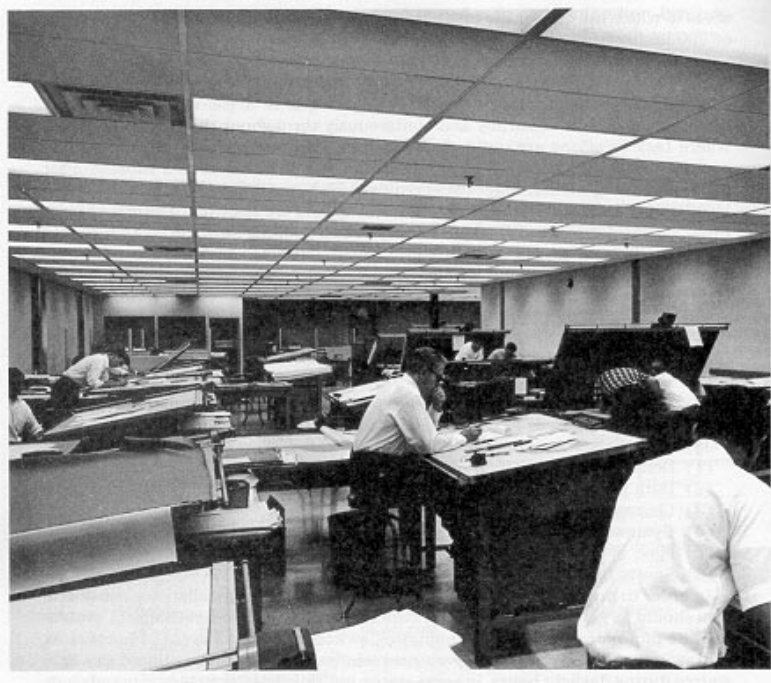
Figure 127—Near-Horizontal Drafting Boards Positioned So That Draftsmen's Views Are Parallel with the Luminaires
